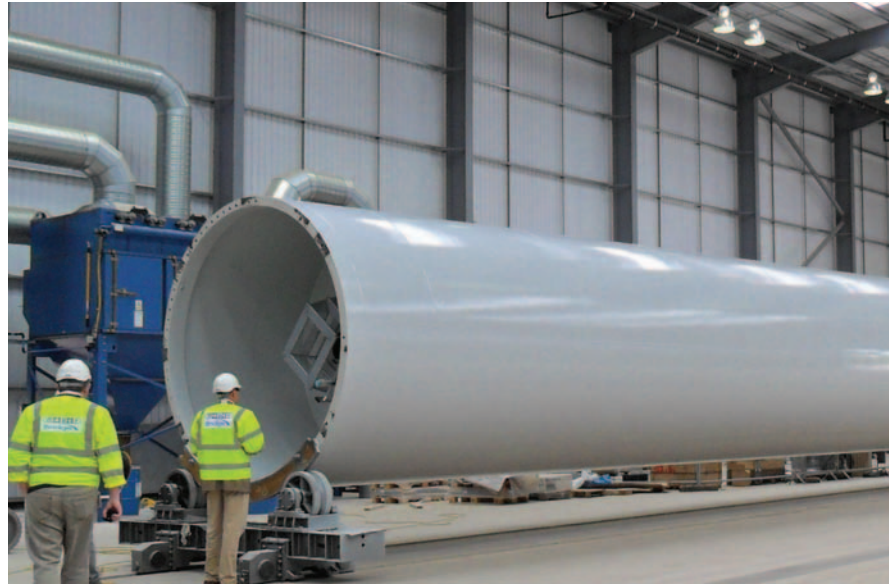
Fabricated turbine towers nearing completion
